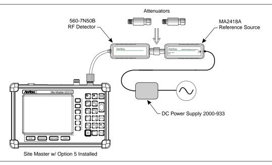
Figure 3. Power Monitor Verification
