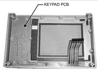
Figure 16. Front Panel Keypad PCB Location
