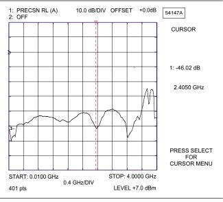
**Figure 6.** Direct Readout of the Precision Return Loss
