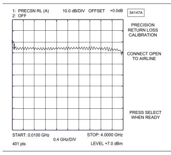
Figure 5. Example of a Good Connection
