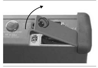
Figure 9. Removing the Battery Access Door
