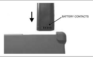
Figure 11. Battery Orientation
