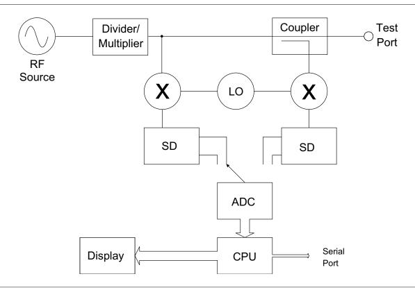
Figure 2. Site Master Block Diagram
