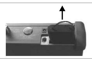
Figure 10. Removing the Battery
