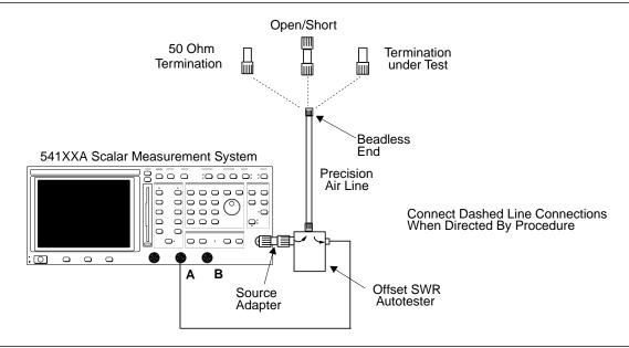
Figure 4. 541XXA Precision Return Loss Setup
