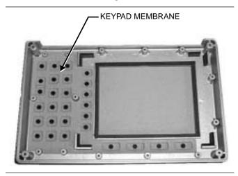
Figure 17. Front Panel Keypad Membrane
