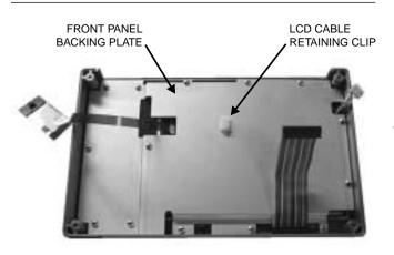
Figure 15. Front Panel Backing Plate
